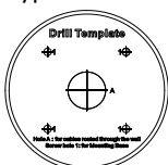
Figure 2-15 Drill Template of the Junction Box
