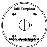
Figure 2-15 Drill Template of the Junction Box
