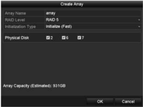
Figure 12. 8 Create Array Interface
