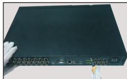
⑥ Install back the cover and secure it with the screws.
