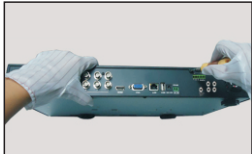
① Loosen the screws on the back.
