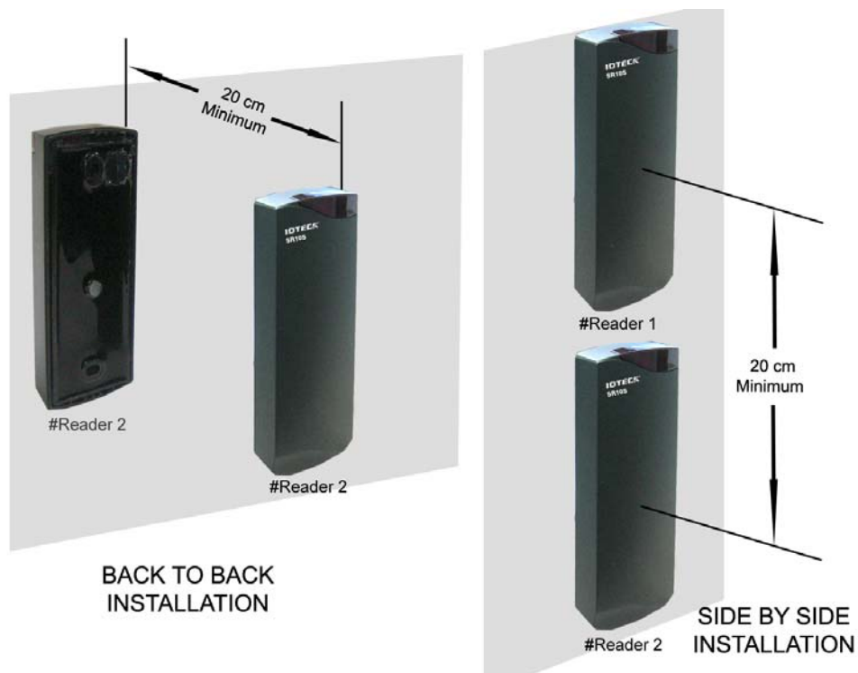
Figure: Minimum Length When Installing More than 2 Readers
