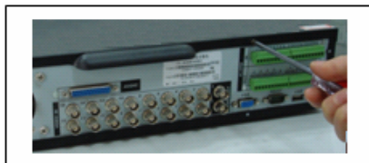
1. Loosen the screws of the upper cover.
