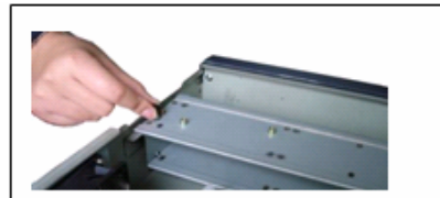
2. Remove the HDD bracket from internal unit.
