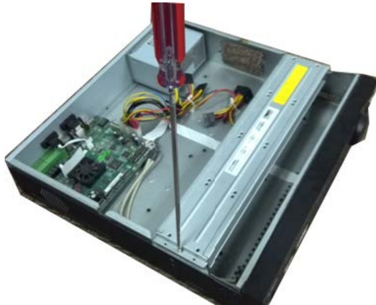
Figure 3-36 Open the top cover
