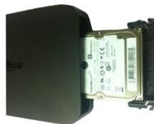
③ Put the HDD into the device
