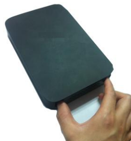
① Draw out the HDD bracket
