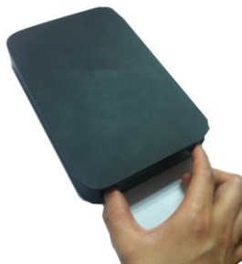
① Draw out the HDD bracket
