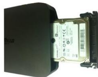
③ Put the HDD into the device
