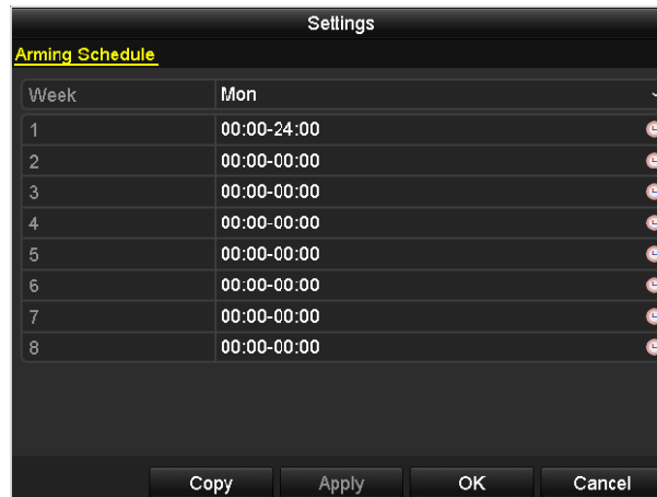
Figure 8. 17 Set Arming Schedule of Alarm Output
