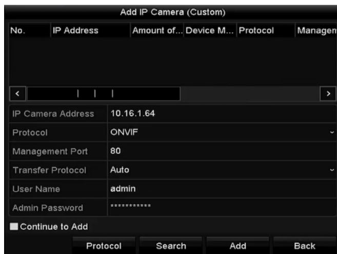
Figure 2.22 Custom Adding IP Camera Interface
