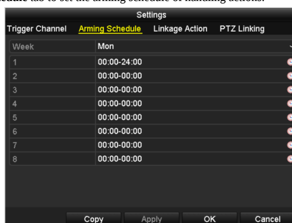
Figure 8.14 Set Arming Schedule of VCA Alarm
