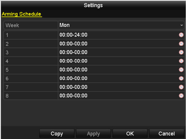
Figure 8. 17 Set Arming Schedule of Alarm Output
