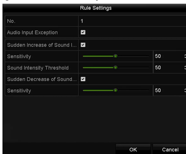
Figure 9.9 Set Audio Exception Detection Rules
