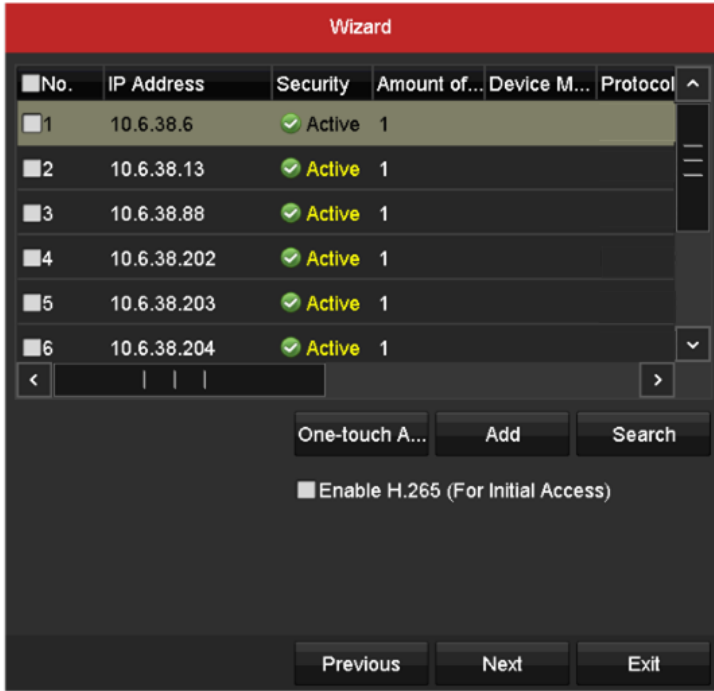
Figure 2. 11 Search for IP Cameras
