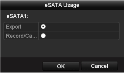
Figure 13. 22 Setting eSATA Usage
