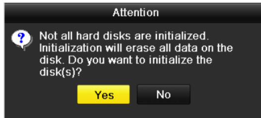
Figure 12. 1 Message Box of Uninitialized HDD
