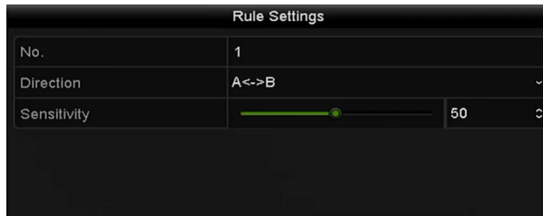
Figure 9. 4 Set Line Crossing Detection Rules
