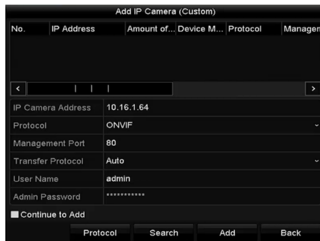
Figure 2. 28 Custom Adding IP Camera Interface
