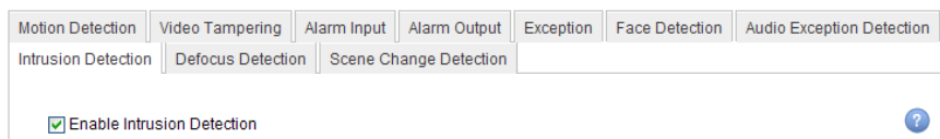
Figure 6. 6 Setting Intrusion Detection on IP Camera
