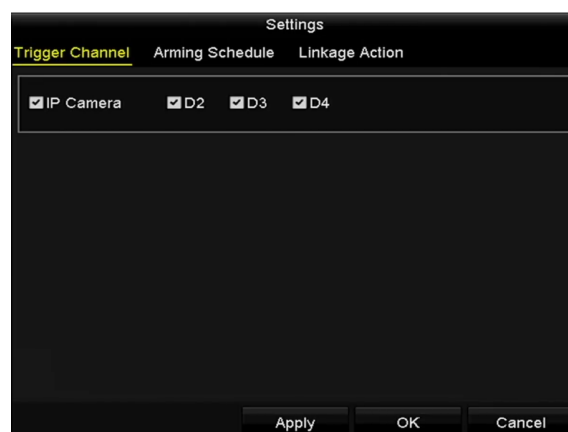
Figure 5.17 Set Trigger Camera of VCA Alarm
