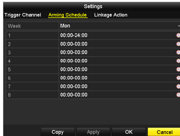
Figure 8.3 Set Arming Schedule of Motion Detection
