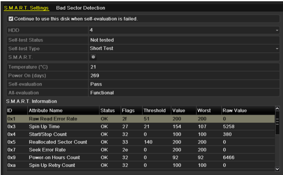
Figure 13. 27 S.M.A.R.T Settings Interface
