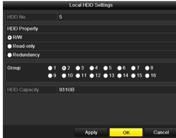
Figure 12-13 Local HDD Settings Interface
