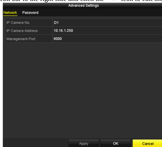
Figure 2. 29 Network Configuration of the Camera
