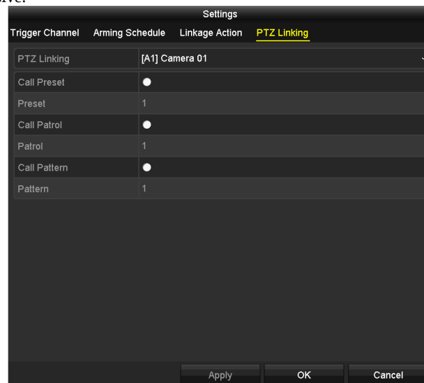
Figure 8. 8 Set PTZ Linking of Alarm Input
