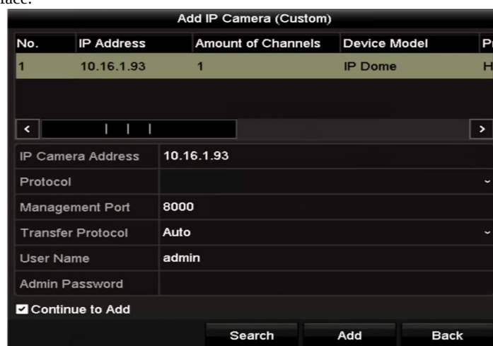
Figure 2.24 Custom Adding IP Camera Interface
