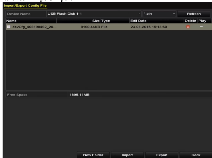
Figure 14. 6 Import/Export Configuration File
