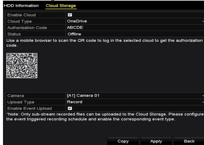
Figure 12. 20 Upload to Cloud Storage Interface
