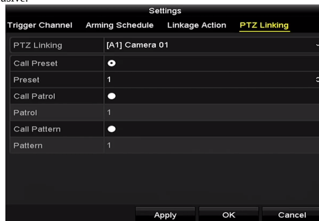
Figure 8.8 Set PTZ Linking of Alarm Input
