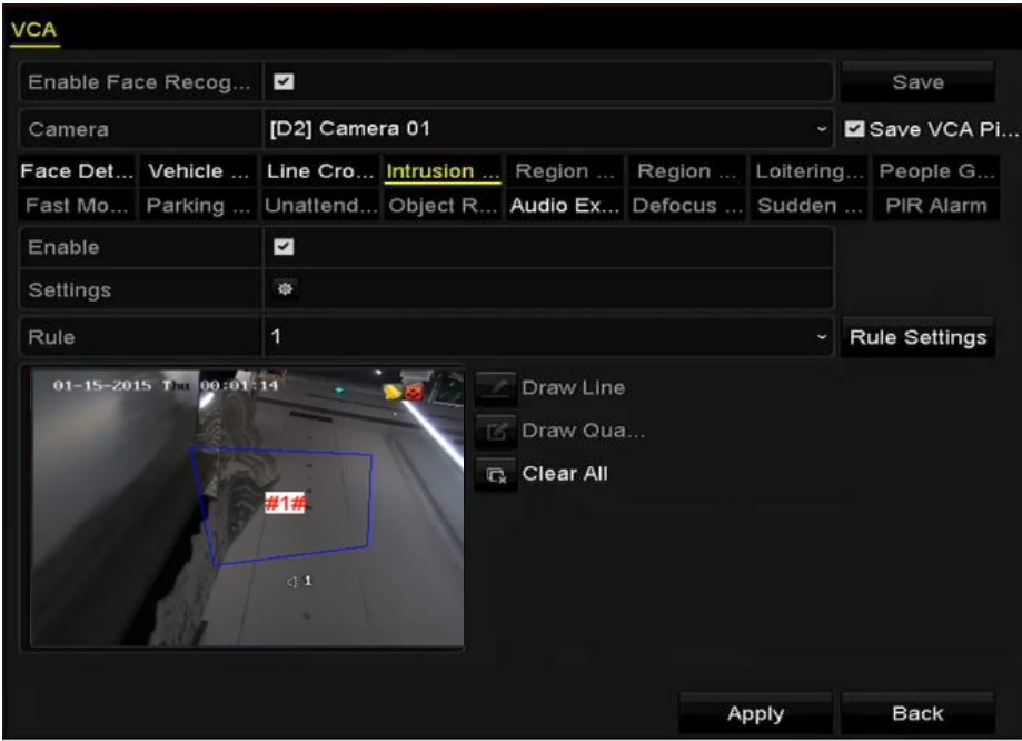
Figure 9. 7 Draw Area for Intrusion Detection
